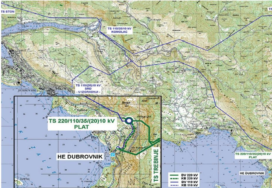
The 220/110/35/20(10) kV substation (SS) Plat is situated at the southern access to the town of Dubrovnik, above the Adriatic main road, near the village of Plat, approximately 800 m north of the present 220 and 110 kV switchyard of the Dubrovnik hydro power plant.
